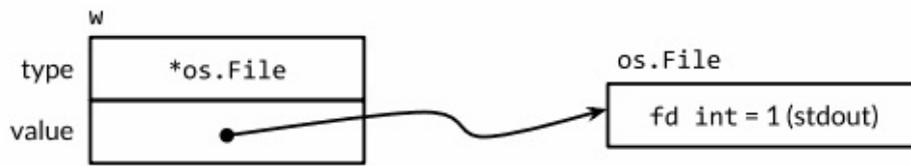
Figure 7.2. An interface value containing an `*os.File` pointer.
