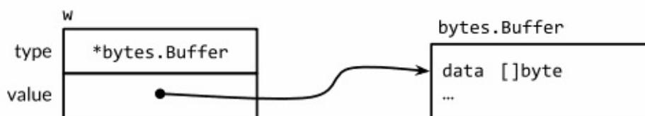
Figure 7.3. An interface value containing a `*bytes.Buffer` pointer.
