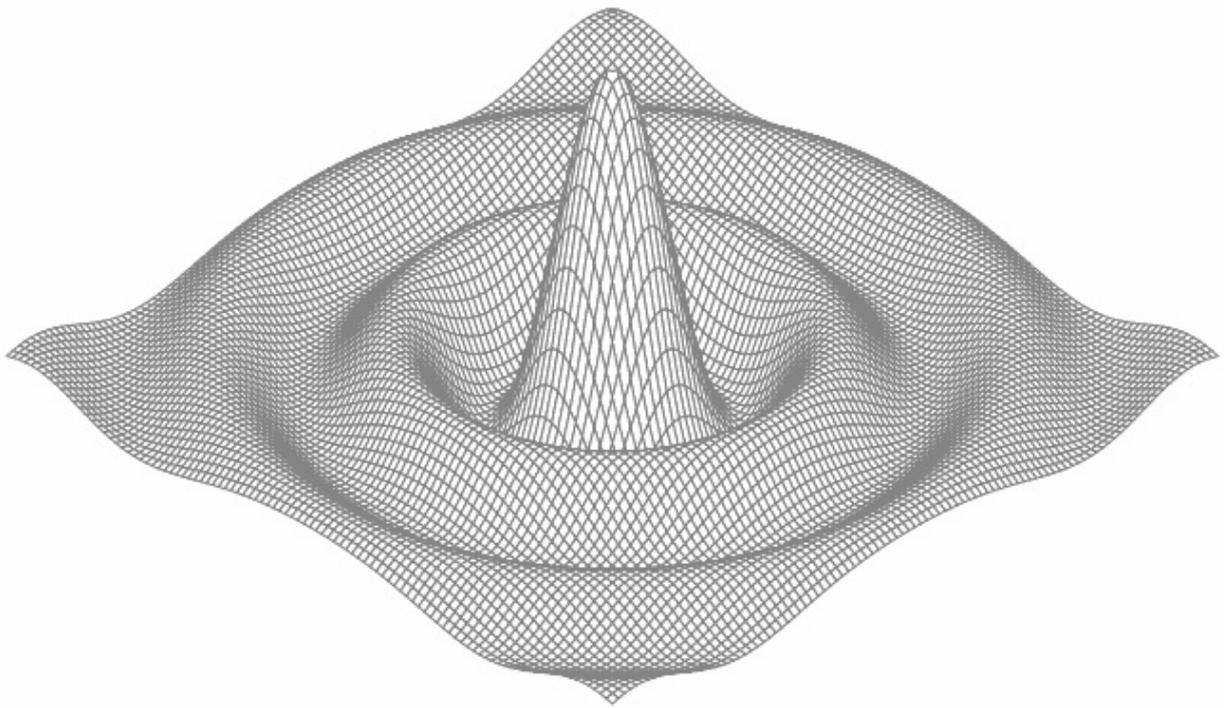
Figure 3.1. A surface plot of the function  $\sin(r)/r$ .
