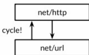
Figure 11.1. A test of `net/url` depends on `net/http`.
