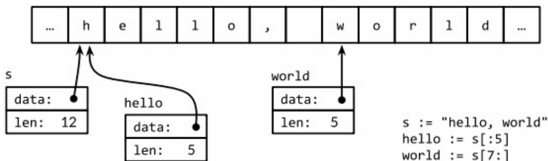
Figure 3.4. The string "hello, world" and two substrings.
