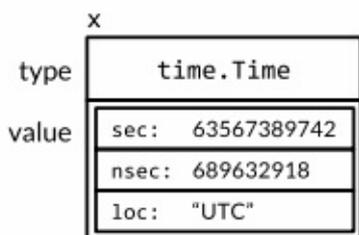
Figure 7.4. An interface value holding a time.Time struct.
